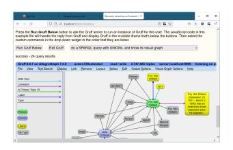
A Gruff feature allows a single launcher instance of Gruff to be running as a server and listening for requests from web browsers. It will launch a separate instance of Gruff for each web page that requests one, up to a specified limit. It can
